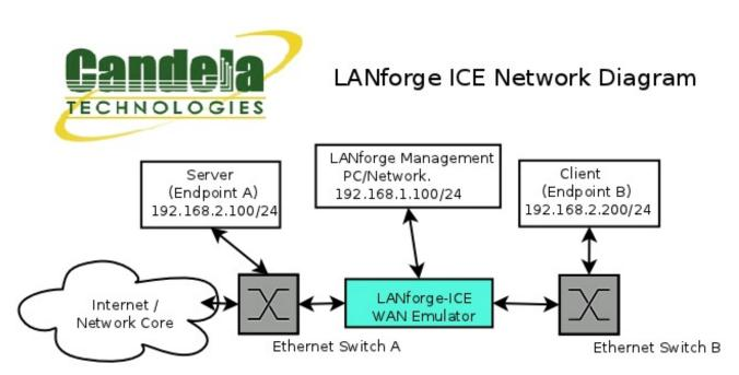
This diagram shows how one might use LANforge ICE to emulate a Wide Area Network between a Server and Client. When the Client communicates with the Server, the traffic will flow through the Ethernet switches and then through LANforge ICE. LANforge ICE will enforce the rate limitation and other network emulation as configured. The Client and Server are on the same subnet. For a simpler configuration, the Client and Server can be directly connected to the LANforge ICE system.
