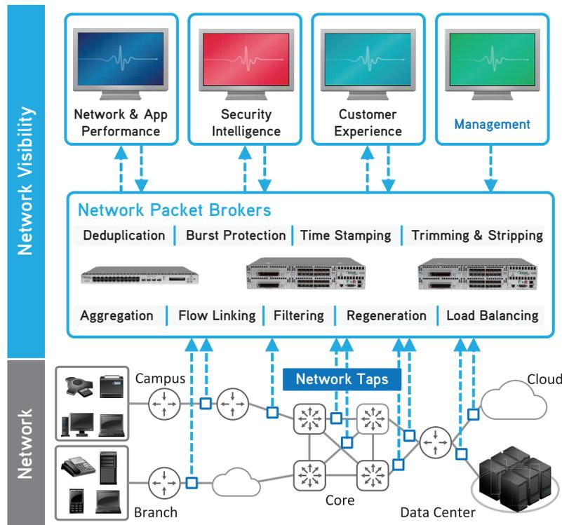
The Network Visibility Framework provides a simple, scalable approach using management features that can integrate into existing work-flow processes and global network management systems (NMS).
