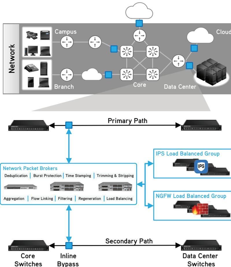
Even better, employing Ixia's Inline Security Framework gives you the ability to load balance traffic between multiple security tools. If one security tool fails, it is possible to automatically rebalance traffic among the remaining tools to maintain security operation.
