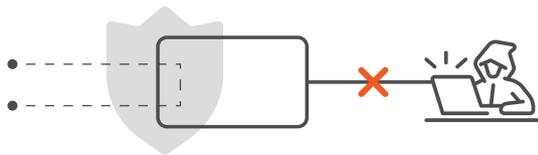
IOTA's In-line circuit is isolated from the other interfaces, internal storage and analysis processing. This makes sure your network stays safe from outside attacks while still enabling full network visibility and analysis.
