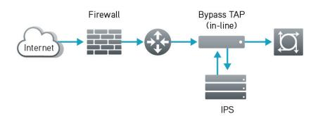
Because of its location in the network, the bypass tap has specific requirements placed upon it that include the following:
