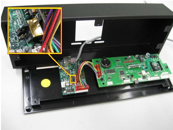
Figure 2-5: Installing the Jumper to Activate Factory IP Address
